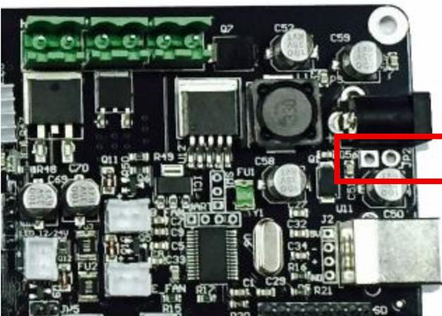
If you use the power adapter, the switch can be connected in both holes. If the switch is not used then use the available short connection else, the board will not get energized and will not work.
